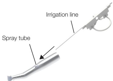
5. Connect the irrigation line to the spray tube of a handpiece (straight or contra-angle).
