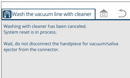
\* If the
