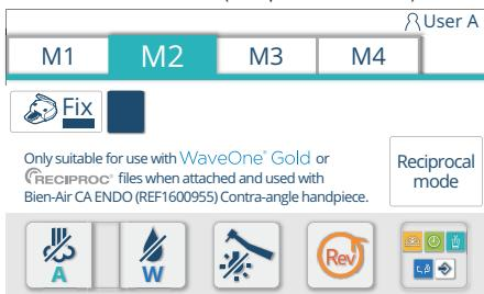
A buzzer sounds, and the micromotor screen (reciprocal mode) appears. Setting of the reciprocal mode is memorized in the starting condition after powering on.
