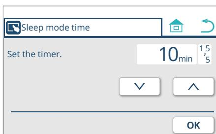
5. Press the and switches to select one of three durations ('5 min,' '10 min,' and '15 min').
