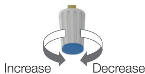
All the knobs decrease the flow rate when turned clockwise and increase it when turned counterclockwise.
