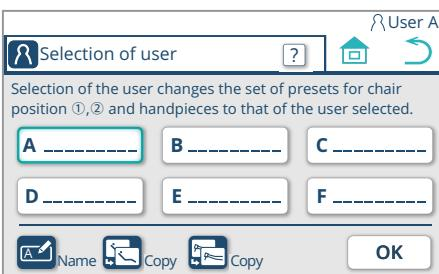
2. On the "Selection of user" screen, press the switch. The "Structure for Patient and User" screen is displayed.
