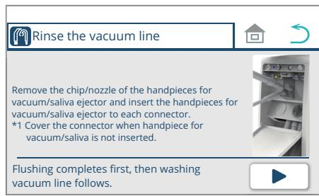
\* To stop washing the vacuum line in progress, press the switch.
