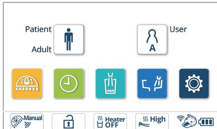
Press the function switch
