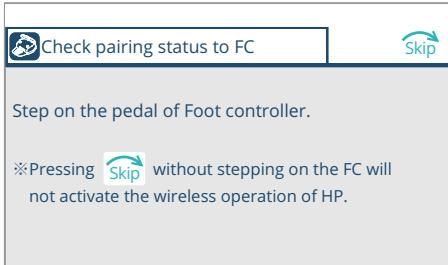
Hold down the pedal of the wireless foot controller until the flushing screen appears.
