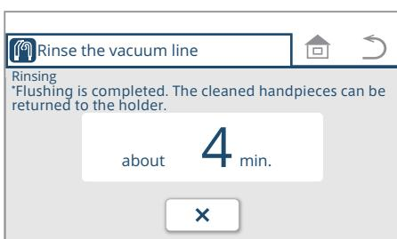
\* To stop rinsing the vacuum line in progress, press the
