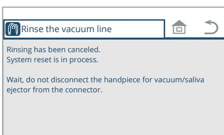
\* If the
