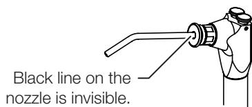
There is no gap between the inner part and outer ring of the nozzle detaching lever
