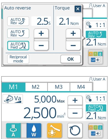
4. Select automatic forward function **AUTO Fwd** from the automatic reverse function / automatic forward function setting
