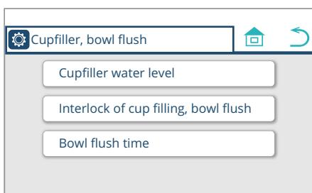
4. Press 'Cupfiller water level.' The Cupfiller water level setting screen appears.
