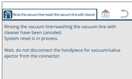
\* If the switch is pressed during washing, the screen shown in the left figure appears.
