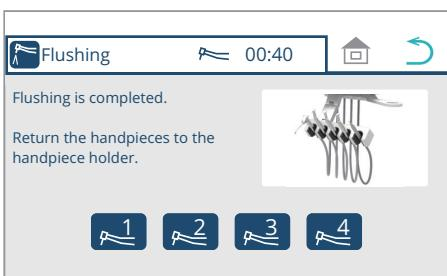
7. Once flushing is completed, return the handpiece to the instrument holder. When the handpiece is returned, the home screen appears.
