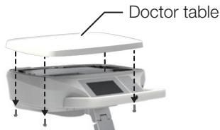
2. Remove the seven screws and detach the table top.
