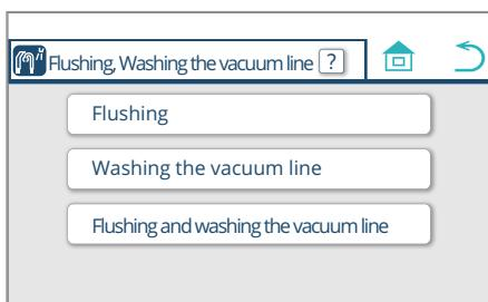
3. Press the 'Washing the vacuum line' switch.
