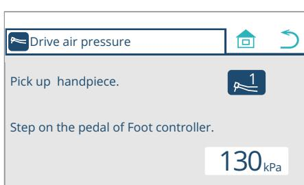
4. Pick up the handpiece to measure the pressure from the instrument holder.
