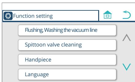
If the washing function for vacuum line is not equipped, 'Flushing' appears on the screen instead.
