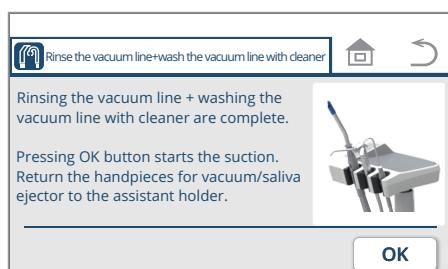
3. When you have finished rinsing the vacuum line+washing the vacuum line with cleaner, press the switch.
