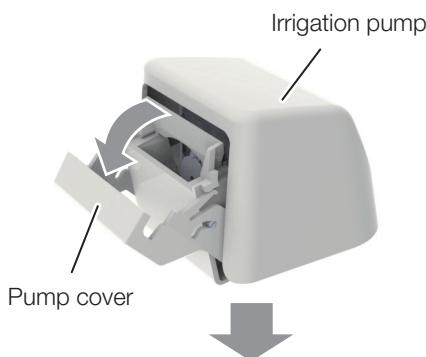
6. Open the pump cover. Attach the cassette of the irrigation line to the irrigation pump.
