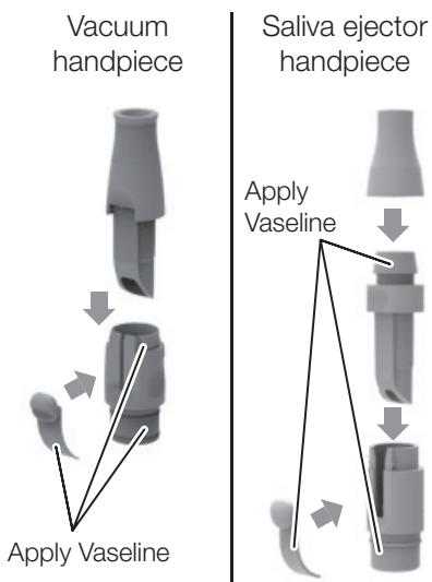
After autoclave sterilization, disassemble the handpieces, apply Vaseline, and reassembly before use.
