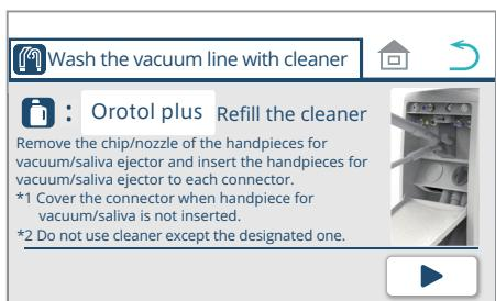
\* If the amount of cleaner is insufficient, the screen shown in the left figure appears. Refill the cleaner.
