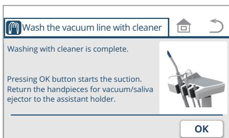
3. When you have finished washing the vacuum line with cleaner, press the
