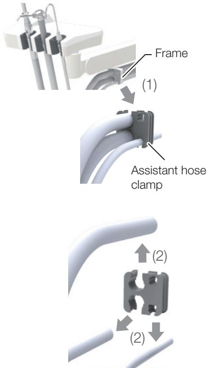
Assistant hose clamp of the assistant unit is detachable from the frame, which is suitable for cleaning.
