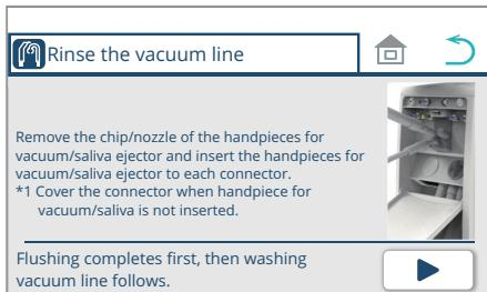
6. Open the front panel of the cuspidor unit. Pick up the vacuum and saliva ejector handpieces from the assistant holder and insert them into the connector.
