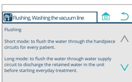
Explanation of flushing and washing the vacuum line
