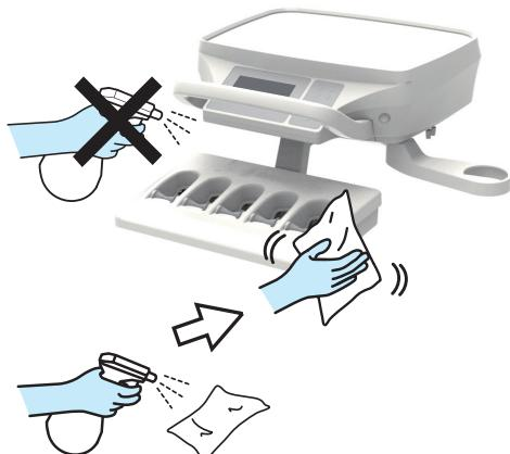
Do not use a brush or scrubber during maintenance. All of these may leave scratches and/or ingrained dirt.
