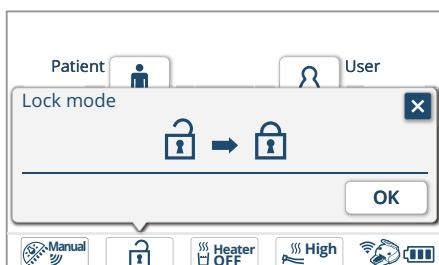
1. Open the [Lock mode] screen, and press **OK**.
