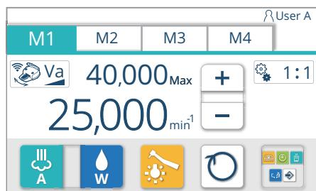
When the micromotor is picked up from the instrument holder, the micromotor screen is displayed.
