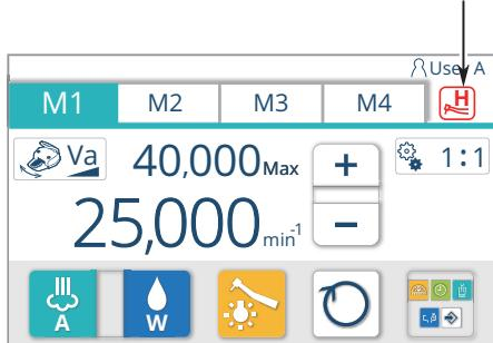
If the product is used for a long time at a high load, the overheating prevention function is activated and the torque is automatically decreased, in order to prevent the micromotor unit overheating. If this occurs, a buzzer sound is heard, and **H** is displayed. While this indication is displayed, the overheating prevention function is activated.
