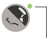
When the headrest function is selected, the lamp is turned on
