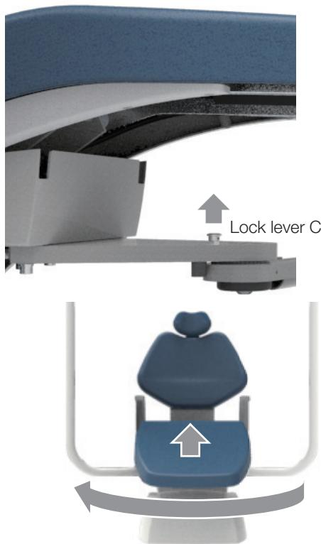
2. Pull up the lock lever C on the swing arm bracket to unlock.
