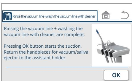
3. When you have finished rinsing the vacuum line+washing the vacuum line with cleaner, press the
