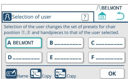
In this example, the name “BELMONT” has been entered. The registered name is indicated for the User memory A box and displayed at the top right.
