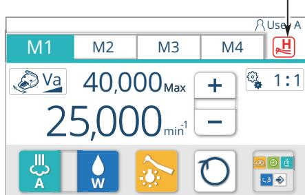
If the product is used for a long time at a high load, the overheating prevention function is activated and the torque is automatically decreased, in order to prevent the micromotor unit overheating. If this occurs, a buzzer sound is heard, and **H** is displayed. While this indication is displayed, the overheating prevention function is activated.
