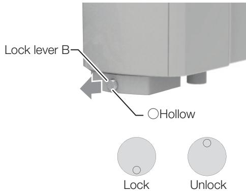
5. Pull forward the lock lever B on the bottom of the cuspidor unit until the red mark is seen, then turn the lock lever B so the hollow comes to the upside position.
