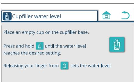
5. Place an empty cup on the cupfiller base, and press and hold the
