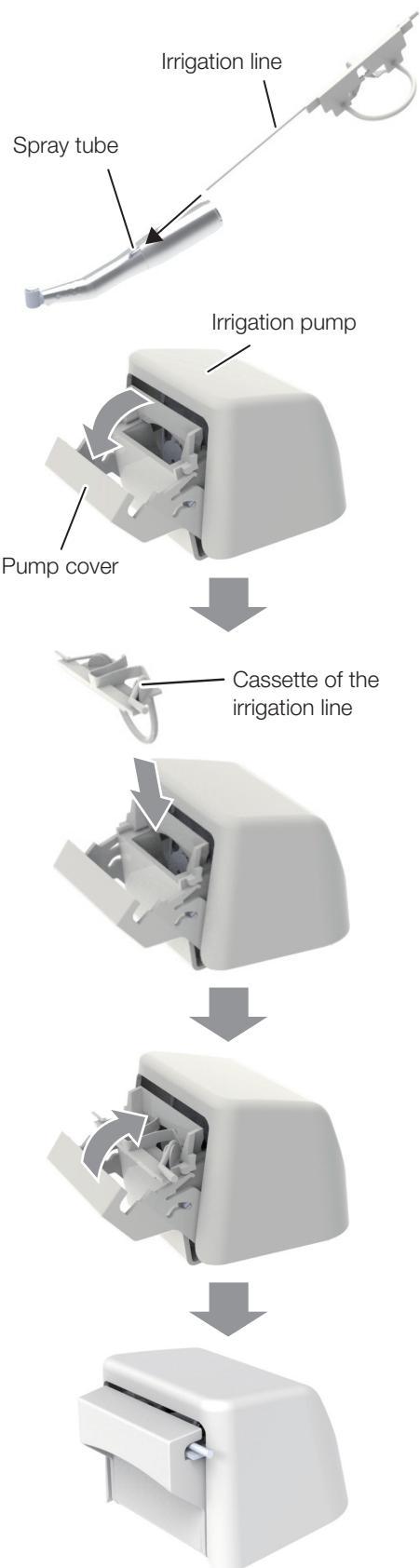
5. Connect the irrigation line to the spray tube of a handpiece (straight or contra-angle).
