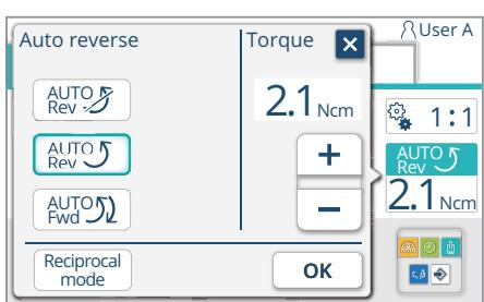
4. Select the required automatic reverse function / automatic forward function setting
