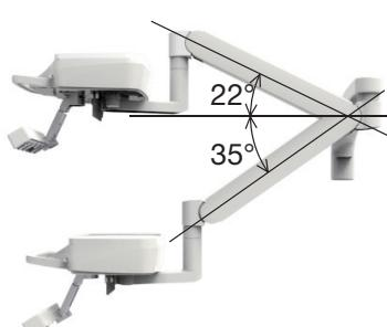
Moving the doctor table upward/downward without releasing the brake may cause damage to the product.
