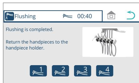
7. Once flushing is completed, return the handpiece to the instrument holder.
