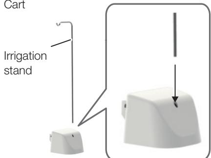
2. Insert the irrigation stand into the hole on the back of the pump cover.
