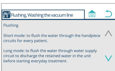
Explanation of flushing and washing the vacuum line
