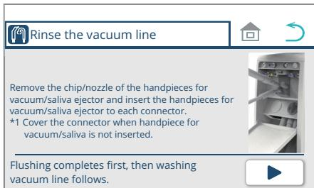
6. Open the front panel of the cupidor unit. Pick up the vacuum and saliva ejector handpieces from the assistant holder and insert them into the connector.
