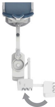
10. Switch the position of the assistant holder to the other side. At that time, the vacuum hose and saliva ejector hose will twist. Pick them up from the assistant holder to remove the twist.
