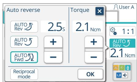
4. Select automatic forward function **AUTO Fwd** from the automatic reverse function / automatic forward function setting
