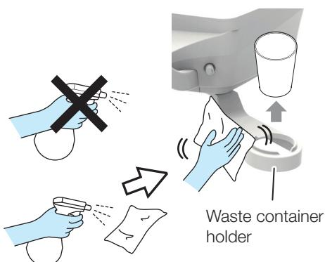
When the waste container becomes full, replace a paper cup for the waste container holder.
