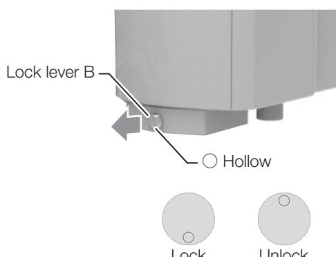
7. Pull forward the lock lever B on the bottom of the cuspidor unit until the red mark is seen, then turn the lock lever B so the hollow comes to the upside position.
