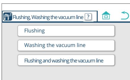
3. Press the 'Flushing and washing the vacuum line' switch.
