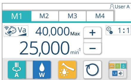
Memory can be selected from four memories (M1 to M4). The memories can be toggled by pressing the memory tab.
