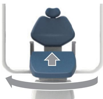
2. Lift the toe board of the seat cushion and swing the light pole to the other side as shown on the left figure.
