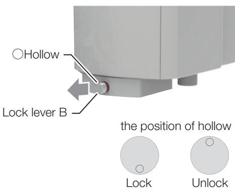
11. Turn the lock lever B so the hollow comes to the downside position.
