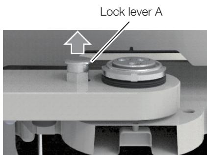
8. Remove the swing bracket cover by pulling in the direction of the arrow. Pull up the lock lever A and turn it until the lever is locked in place.
