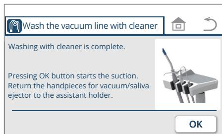
3. When you have finished washing the vacuum line with cleaner, press the
