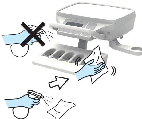
Do not use a brush or scrubber during maintenance. All of these may leave scratches and/or ingrained dirt.
