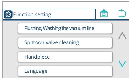
3. Press the 'Flushing' switch.
