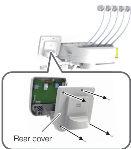
2. Detach the button battery (CR1632) on the PCB.
