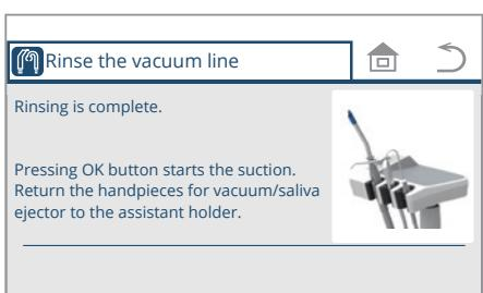
After the suction starts, remove the vacuum and saliva ejector handpieces from the connector.
