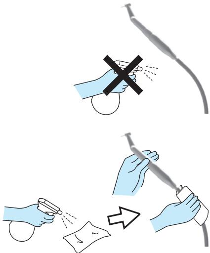
Do not spray detergent directly onto the exterior.
