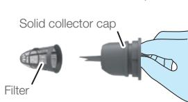
4. Wash the solid collector cap and the filter under running water.
