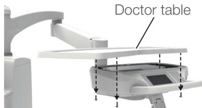
1. Remove the four screws under the doctor table and detach the doctor table.
