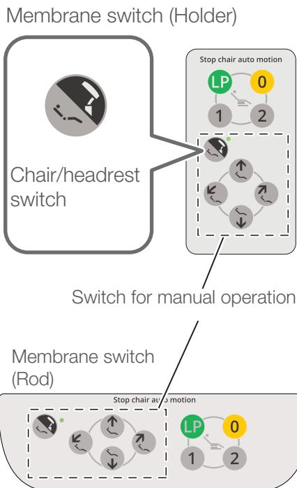
By holding down the chair/headrest switch
