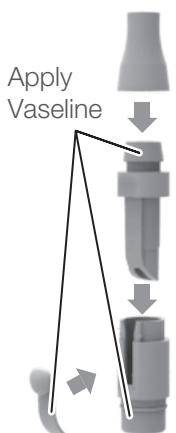
After autoclave sterilization, disassemble the handpieces, apply Vaseline, and reassembly before use.
