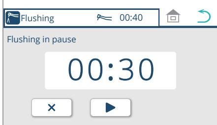
\* To resume flushing, press the switch.
