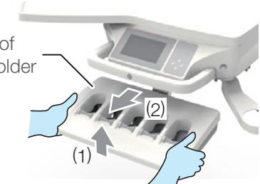
1. Hold the upper part of the place holder with both hands and pull it upward slightly. (1)
