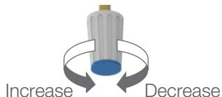
All the knobs decrease the flow rate when turned clockwise and increase it when turned counterclockwise.
