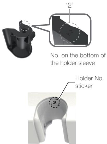
Each holder sleeve has its No. on the bottom, and a sticker showing the same No. is attached to the assistant holder. Make sure you attach the holder sleeve to the holder with the same No.
