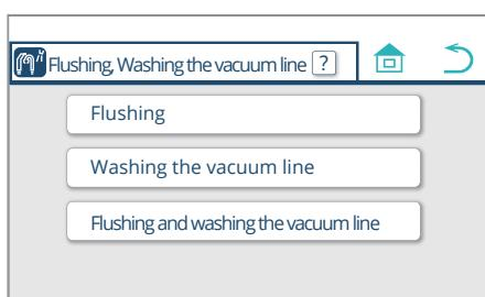
3. Press the 'Flushing' switch.
