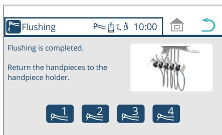
7. After rinsing of the vacuum line is completed, return the handpieces for doctor unit to the instrument holder.
