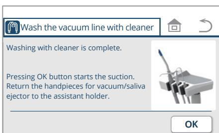
3. When you have finished washing the vacuum line with cleaner, press the
