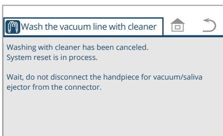
\* If the
