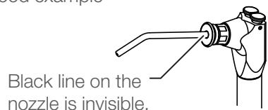
There is no gap between the inner part and outer ring of the nozzle detaching lever
