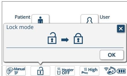
Call the “Lock mode” screen and press **OK** to lock the operation.
