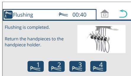
7. Once flushing is completed, return the handpiece to the instrument holder.
