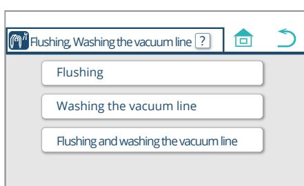
3. Press the 'Flushing' switch.
