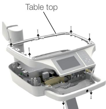
2. Remove the seven screws and detach the table top.
