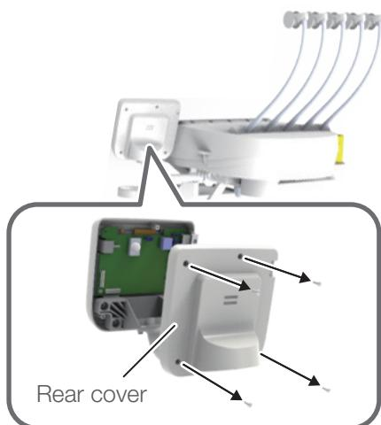
2. Detach the button battery (CR1632) on the PCB.
