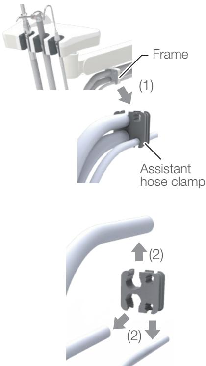
Assistant hose clamp of the assistant unit is detachable from the frame, which is suitable for cleaning.
