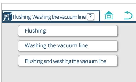
3. Press the 'Flushing' switch.
