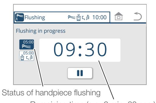
If the cuspidor bowl is not equipped, rinsing the vacuum line starts 5 minutes after flushing the water circuits of handpieces.
