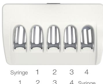
All the knobs decrease the flow rate when turned clockwise and increase it when turned counterclockwise.
