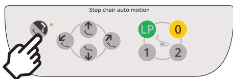
1. Move the seat of the chair and backrest to the desired position using the manual control switch or preset switch on the control panel. (The stick switch for manual/automatic operation can also be used to do the same.)
