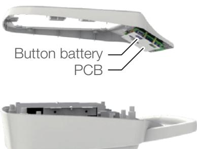
3. Detach the button battery (CR1632) on the PCB.
