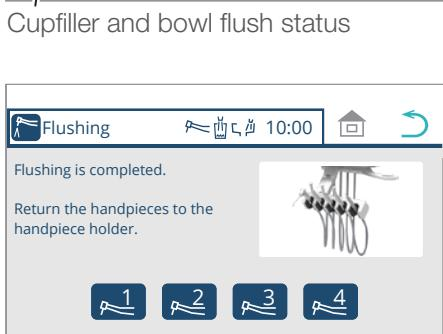
7. Once flushing is completed, return the handpiece to the instrument holder.
