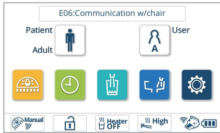
When turning off the chair, "E06: Communication with chair" is displayed on the touch panel because of the interruption of communication between unit and chair, then LED indicator of the cuspidor unit lights up in orange, which is not malfunction.
